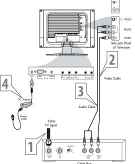
The AUDIO and VIDEO In jacks on the connections of other equipment. Connect a VCR, DVD Player, Video Game, Camcorder, etc., to these jacks. To view the material playing on the other equipment, set the LCD TV to its AV Mode.
